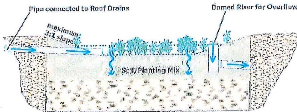
Figure 4: Cross-Section of Typical Rain Garden/Bioretention Area
